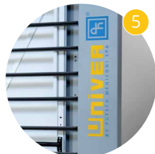
5 Univer dust catcher for horizontal cuttings (TRK) Conductor de polvo Univer para cortes horizontales (TRK)
